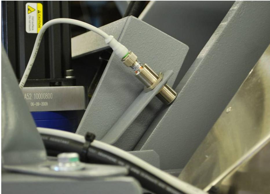
Figure 17 - Press Arm Proximity Switch Alignment
