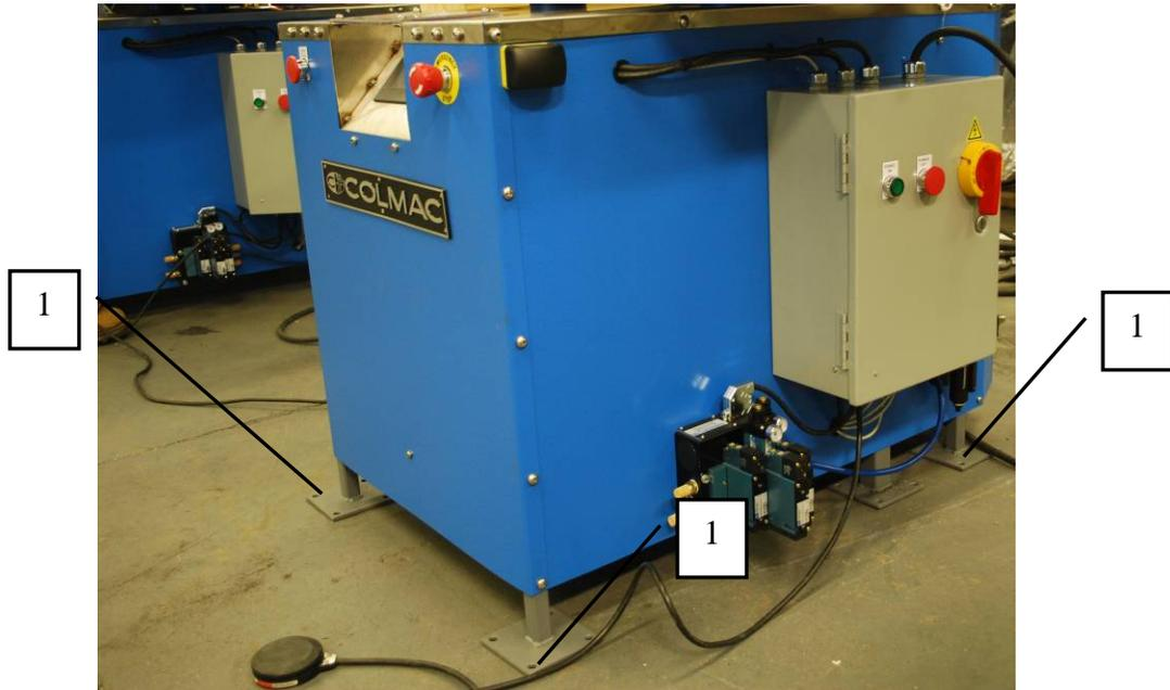
Figure 1 – Installation Bolt Holes
