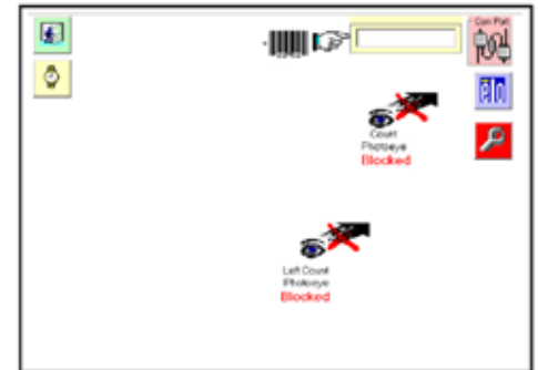
The maintenance screen displays real-time status of sensors and tests bar code reader integrity.
