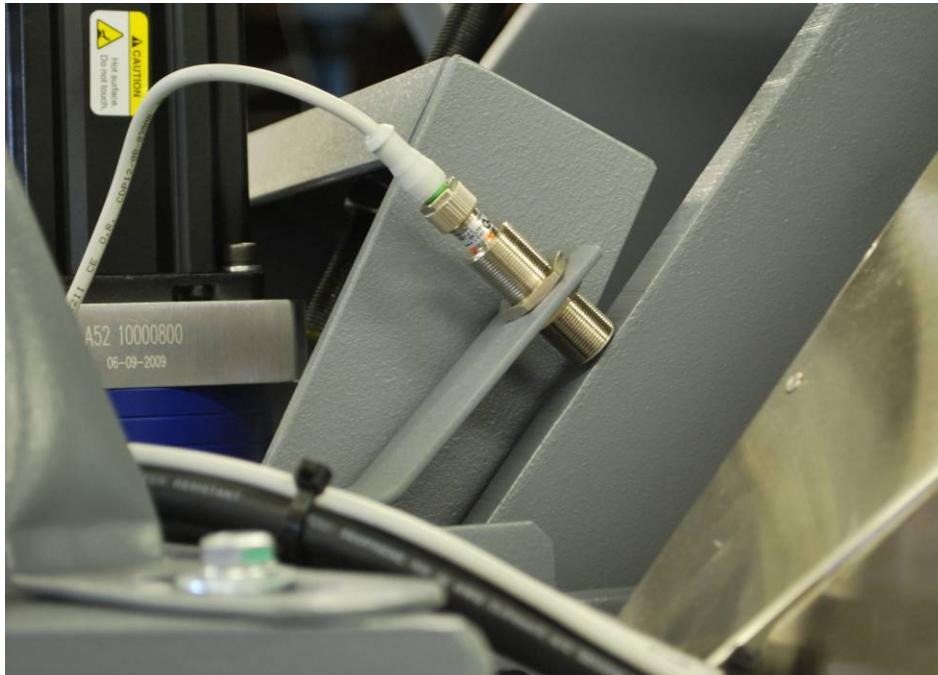
Figure 17 - Press Arm Proximity Switch Alignment
