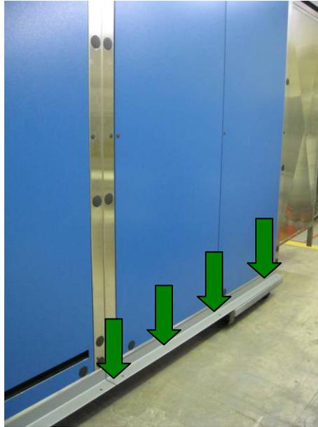
Figure 1 - Tunnel Leveling Pad
